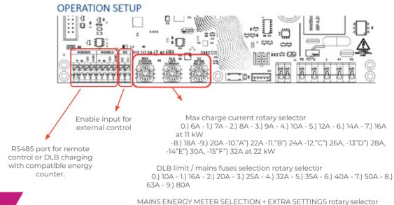
O.) DLB DISABLED, use standard charge preset to »MAX CHARGE CURRENT«
